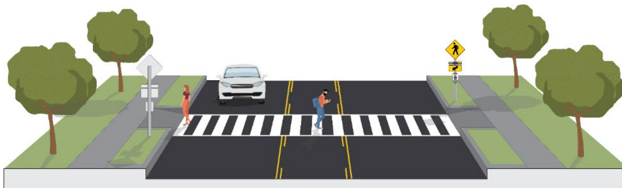
Figure 25. Rectangular Rapid Flashing Beacon (RRFB)
